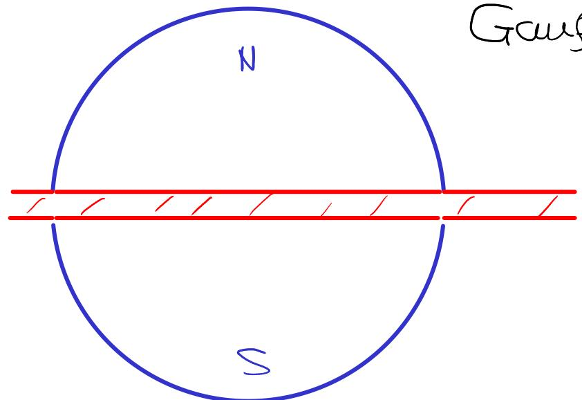
when we pull the hemispheres apart just a tiny bit we add the field in the gap to the set up, consider everything else unchanged. Then we are adding a cylinder to the sphere with a field  $E$
